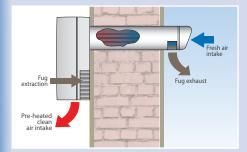
Tubular heat exchanger with separate flows
